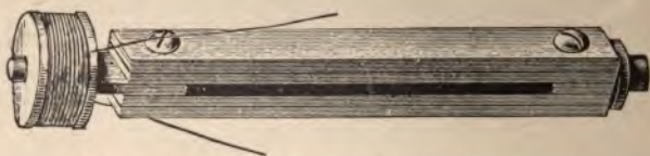
FIG. 66.—Single-pole compound bar telephone magnet.
